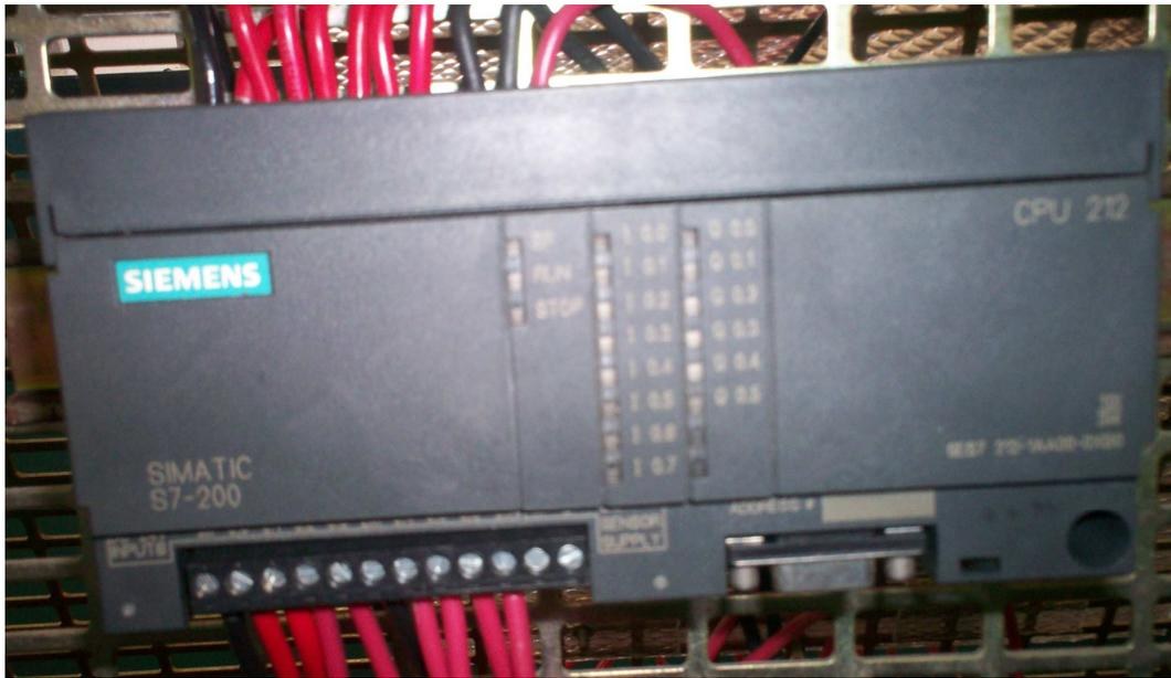
**Figura 4.11:** PLC Siemens S7-200 CPU 212
