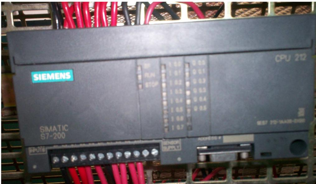
Figura A-5: PLC Siemens S7-200 CPU 212
