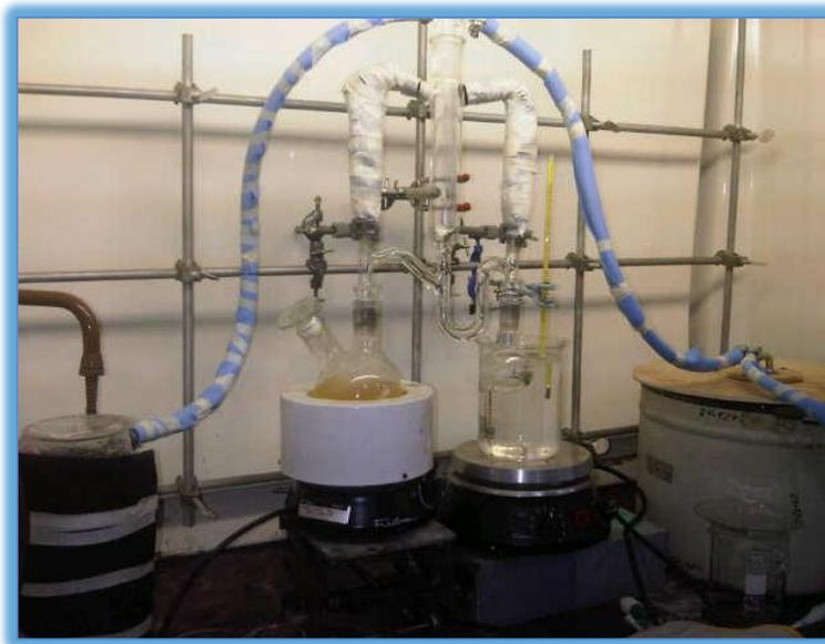
**FIGURA 4.1. MONTAJE DE LA EDS (LIKENS Y NICKERSON, 1964)**
